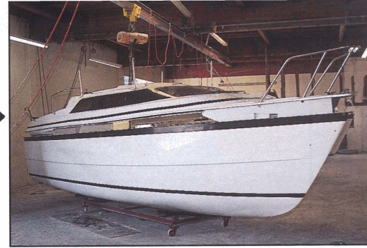
The hull and deck are joined with 3/16" bolts on 4" centers. Top grade adhesive is used to insure a watertight seal. Many builders use screws or pop rivets for this joint. Bolts are better.
