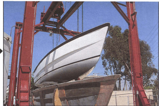
Here the cured hull is being removed from the mold. Notice the high gloss and molded in stripes. All the fiberglass parts are built in precision molds in the same manner as the hull.
