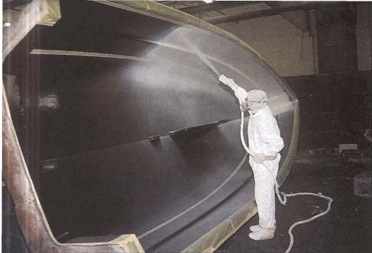
Production begins with the spraying of the exterior color (polyester gel coat) on a highly polished and waxed 3 ton hull mold. The waterline and accent stripes are also sprayed on at this point.
